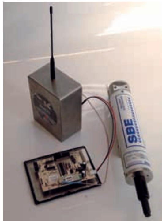
Fig. 2. Detail of the Sea-Bird SeaCat temperature and salinity sensor and the transmitter that were installed onboard the FMC.
